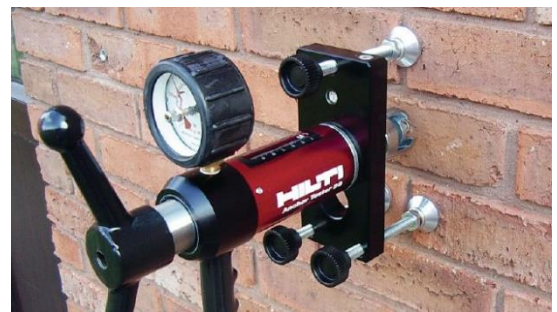
Figure 14 Pull Test equipment - image courtesy of Hilti GB
