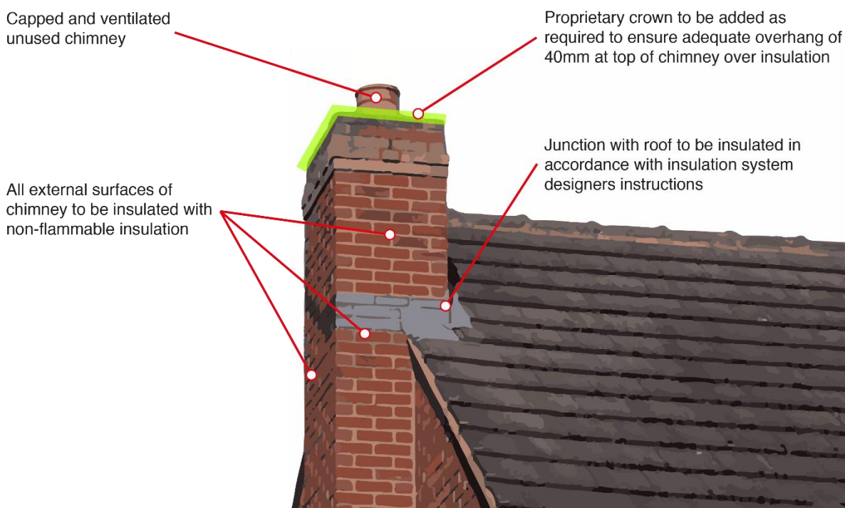
Figure 1 Unused external chimney insulation requirements
